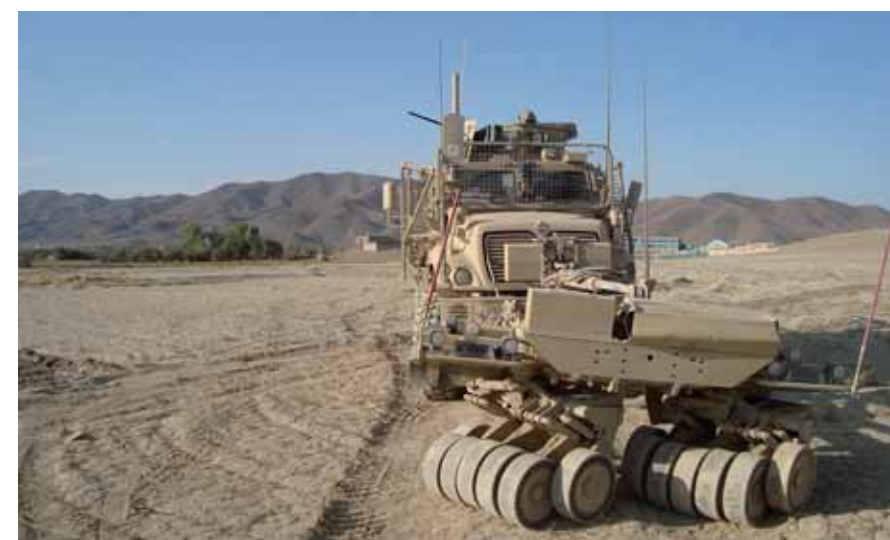
Mine roller, a specialised vehicle used for RCP
